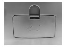
2. Tighten the tailgate emergency zipper, unlock and open the tailgate.
