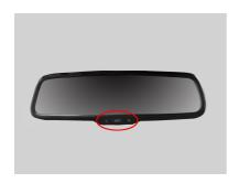
The inner rearview mirror has an anti-glare function, which reduces the reflection from the rear to make the rear view in the best observation state.
