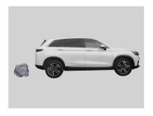
The radar probe cannot detect objects that easily absorb ultrasonic waves such as soft snow, cotton and sponges.
