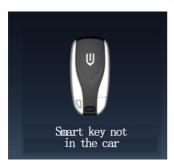
When the smart key is not in the car and the door is closing, the indicator prompts "Smart key is not in the car" for 5s, accompanied by a beep.
