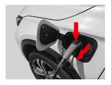
Close the protective cover of the AC charging port, and then close the AC charging port cover.
