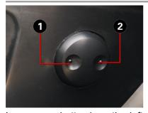
Long press button1 on the left side to support the lumbar. Long press the right button2 to reduce the lumbar support.
