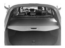
Pull out the cover curtain and clip both sides of the cover curtain into the fixing groove. When the cover curtain is not in use, just remove and retract it.
