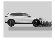
When colliding with easily deformable objects, your safety will not be endangered, so the front airbag will not deploy in such collisions.
