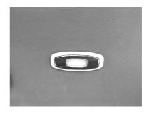
Open the door, the front and rear dome lights will automatically light up and go out after 1 minute, or the whole car will be powered off or locked, and the front and rear dome lights will go out immediately.
