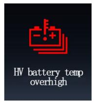
When the temperature of the power battery is too high and the power is reduced, the
