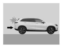
In a rear collision, the head pillowand seat belt will provide you with the best protection, while the front airbag cannot provide significant protection.
