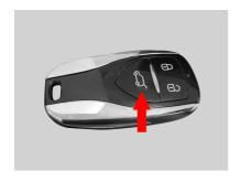
Long press the tailgate opening button on remote control key when vehicle power off;
