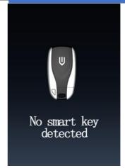
When smart key not detected, the meter will prompt "Smart key not detected" for 5s, accompanied by three beeps. Prompt Message3: Smart key low battery
