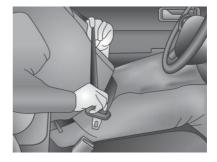
Pull out the seat belt of the shoulder slowly, and make it diagonally across the shoulder, chest, and hip (be carefully not to touch the neck or slip off);
