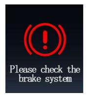
When the Braking system malfunctions, the indicator lights up the malfunction
