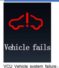
Malfunction light flashes red when running at reduced power, indicator red lights up when the function is disabled at the same time "Vehicle system malfunction" warning 5s, accompanied by loud warning sound.
