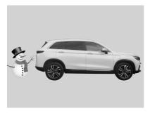
The radar probe may not be able to detect objects higher than the bumper.
