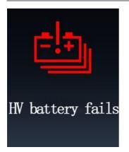
When the power battery malfunctions, the meter flashes (functionally limited)/steady light (emergency shutdown) red indicator at the same time, а "Power battery malfunction" warning is issued for 10s, accompanied by an warning sound.
