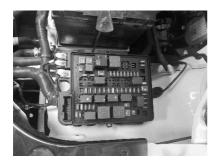
Open the Front cabin, the front fuse box assembly is located on the right side of the Front cabin, press the tabs on both sides to lift the cover to check or replace the fuse.
