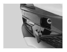
Install the tow hook into the tow hook hole in a clockwise direction, and then tighten it.
