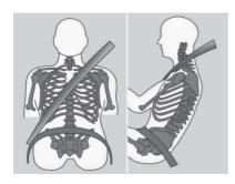
The seat belt is a safety device that ensures that the driver and occupants are restrained in a limited position during a vehicle collision, emergency braking, and sudden steering. We strongly recommend that drivers and occupants wear seat belts correctly at all times to reduce the forward inertia of drivers and occupants caused by collisions, emergency braking and sudden steering. Correct use of seat belts can greatly reduce the casualties of occupants in the vehicle.
