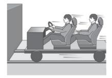
Take the simplest vehicle as an example, suppose that the vehicle is a seat with wheels on which a person can sit. Make it accelerate and then stop, the people in the vehicle will not stop.
