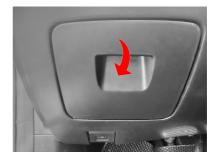
Pull the handle of the storage backwards. and storage box can be opened.
