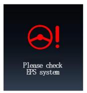
When the electric power steering system is malfunctioning, the meter lights up the malfunction indicator
