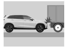
When colliding with the rear of the truck (drilling collision).
