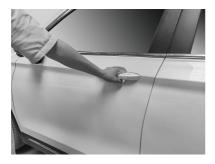
When the vehicle is powered off, bring the key to the front door within about 1 meter and hold the front door handle. After the sensor area inside the front door handle is effectively detected, the door is unlocked.
