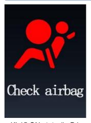
n KL15 ON state (ie D1 mode), when the airbag function fails, the indicator lights up the airbag malfunction indicator
