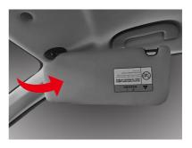
When closing the sun visor, you need to mount the sun visor to the fixed support and push it upward.
