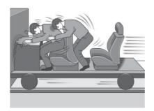
The person continues to move forward until blocked by an object. In actual vehicles, the object may be the windshield or dashboard or seat belt.
