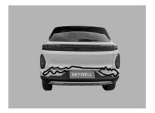
The radar probe is covered by dirt, snow or mud, etc., and may not be able to detect obstacles.
