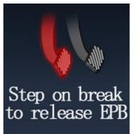
When the electronic handbrake is released without stepping on brake pedal, the indicator will prompt "Please step on brake pedal to release the electronic parking" for 5S, accompanied by a beep.
