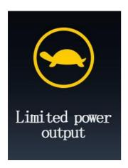
When the battery is insufficient and limited power output, the meter lights up the limp indicator . At the same
