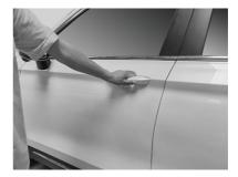
When the vehicle is powered off and there is no key in the vehicle, when all doors (four doors, hood, tailgate) are closed, and the key is within 1 meter of the front door, press the groove on the front door handle to lock the door.
