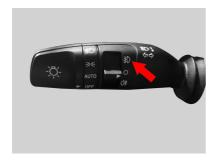
the rear fog light will be turned off; when the low beam is turned off, the rear fog light will be turned off at the same time
