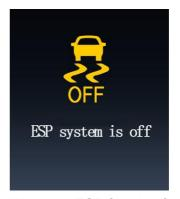
When the ESP function fails or the system is OFF, the indicator lights up the malfunction indicator at
