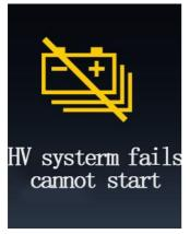
When the high voltage system is cut off and cannot be started.
