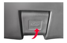
Lift the hood, take out the hood support rod. support the hood at the limit position.
