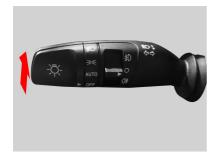
Move the light adjustment handle to the steering wheel and release, the high beam flashes once, and the high beam indicator on the instrument cluster assy flashes
