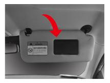
To block the light from the side, you can remove the sun visor from the fixed support and turn the sun visor to the side.
