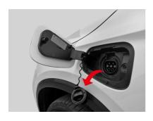
5. Correctly connect the charging gun to the charging port until you hear a "click" sound to lock the charging gun, and the charging connection indicator on the instrument cluster assy will light up.
