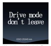
When the vehicle is in D gear or S gear or R gear and the left front door is opened, it will prompt " Driving mode, please leave" for do not 5S. accompanied by three beeps. Prompt Message13: Position is not turned off light warning
