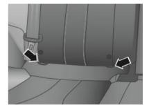
5. Place the seat upright, align the ISOFIX connector of the child safety seat with the corresponding part behind the seat, rotate the ISOFIX handle to push the
