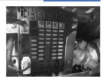
The instrument panel electrical box is located behind the storage box on the lower left side of the instrument.
