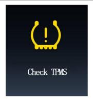
When the tire pressure system is malfunctioning, the meter lights up the malfunction
